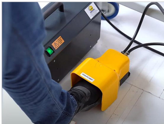
Figure 18: Foot switch for unclamping the workpiece
