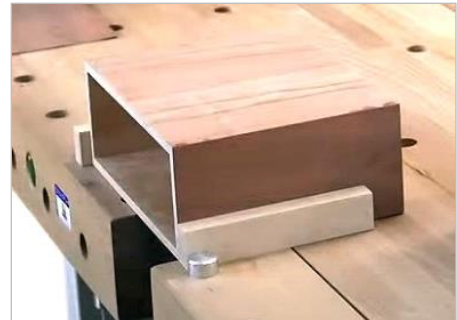
Figure 13: Clamping with waste spacers
