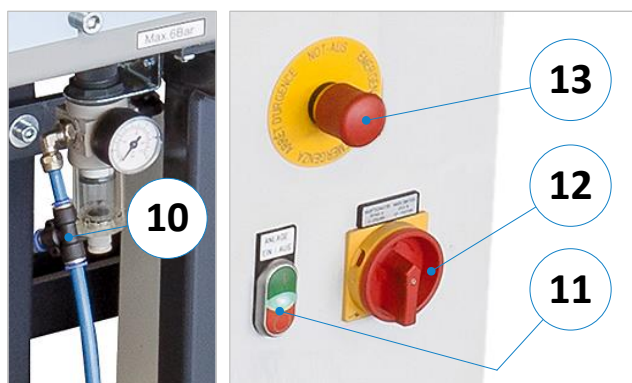
Figure 10: Control switches and compressed air connection
