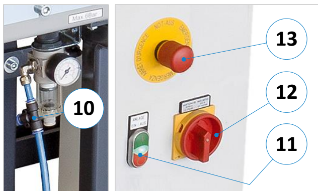
Figure 10: Control switches and compressed air connection
