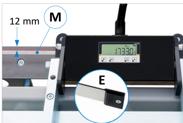
Figure 18: Magnetic tape installation with EXAKT E/KF
