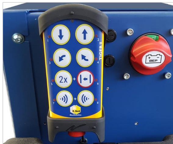
Figure 10: Charging station next to the main switch
