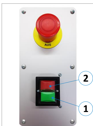
Figure 19: Push-button unit (1.1 - 1.5 kW)
