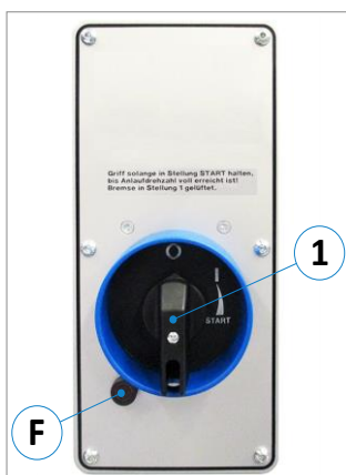
Figure 17: Machine switch (3.0 - 7.5 kW)
