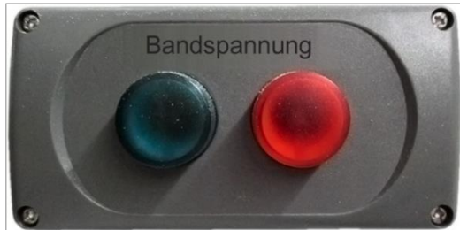
Figure 67: Visual saw blade tension monitoring
