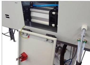
Figure 34: E-stop for feed unit flap
