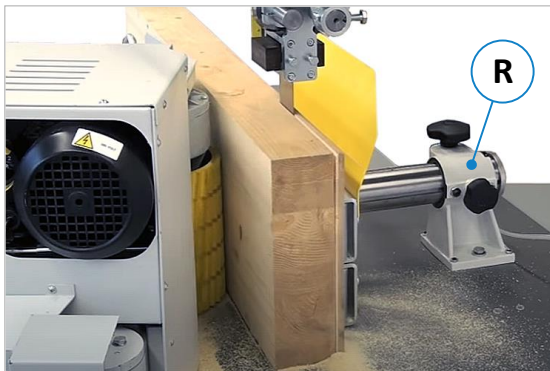
Figure 70: Roller fence and feed unit in use
