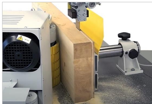
Figure 2: Processing on the band resaw
