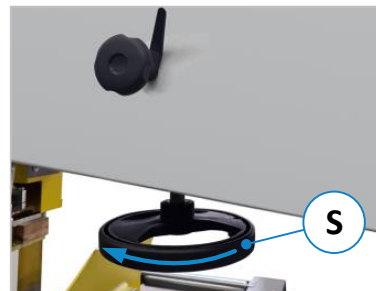
Figure 57: Tension the bandsaw blade
