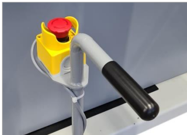
Figure 33: E-stop on foot switch
