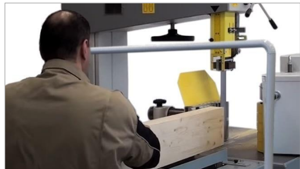
Figure 87: Place the workpiece and guide it to the fence
