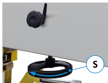
Figure 57: Tension the bandsaw blade
