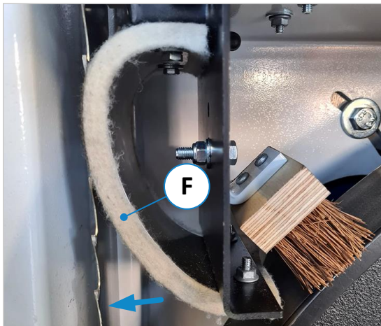
Figure 81: Felt for bandsaw blade lubrication
