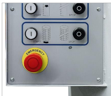
Figure 31: E-stop control panel
