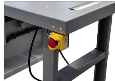
Figure 35: E-stop on removal table
