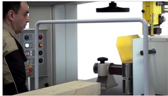
Figure 85: Switch on bandsaw drive and feed unit
