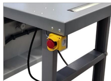
Figure 35: E-stop on removal table
