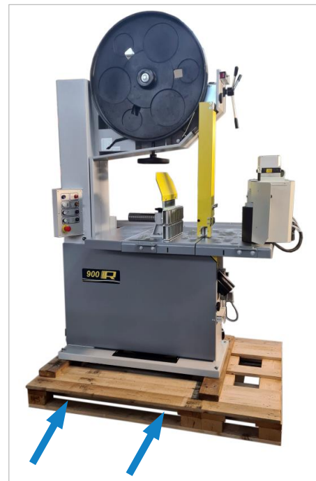
Figure 9: Transporting the machine
