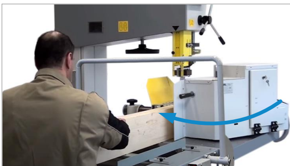
Figure 88: Swivel in the feed unit for machining
