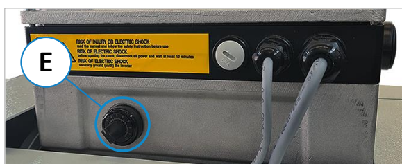
Figure 80: Setting wheel for variable feed rate
