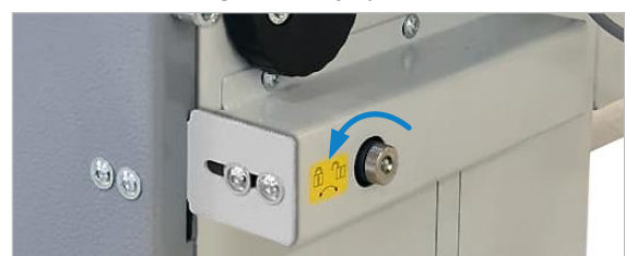
Figure 45: Safety switch - door locked
