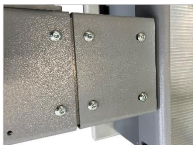
Figure 50: Bridge plate mounted
