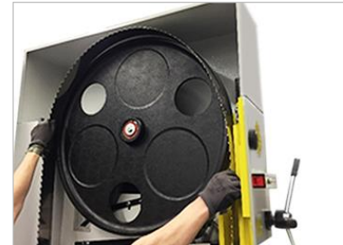
Figure 55: Insert saw blade (top)
