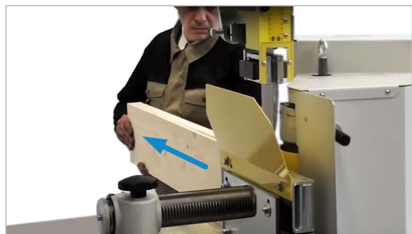
Figure 89: Remove workpiece parts on the removal side
