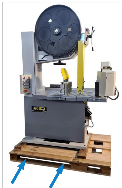
Figure 9 : transport de la machine
