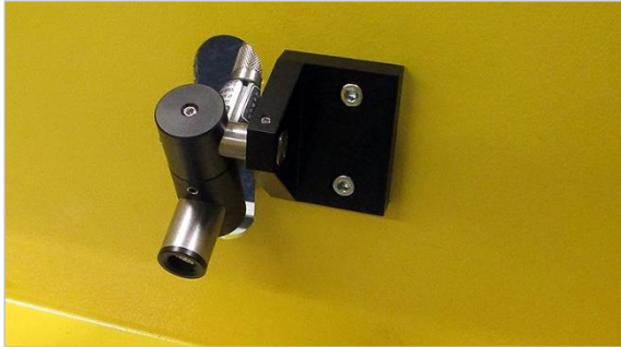
Figure 44: laser unit to indicate the cutting line
