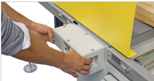
Figure 24: two-hand safety control
