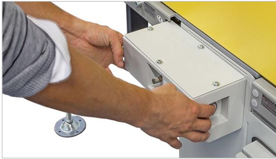
Figure 43: cut triggering via two-hand control
