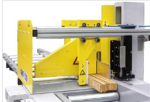
Figure 38: pneumatic horizontal clamping device
