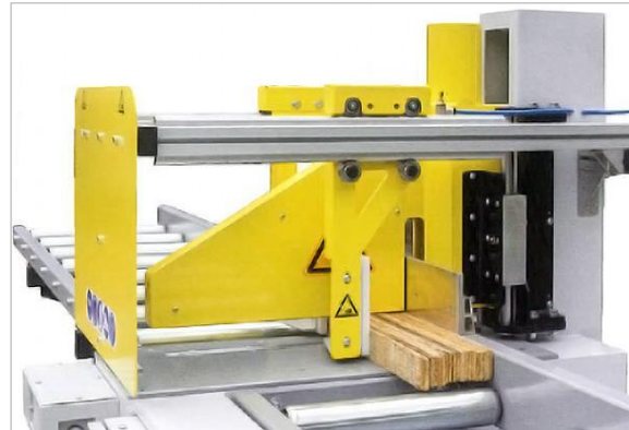
Figure 38: pneumatic horizontal clamping device
