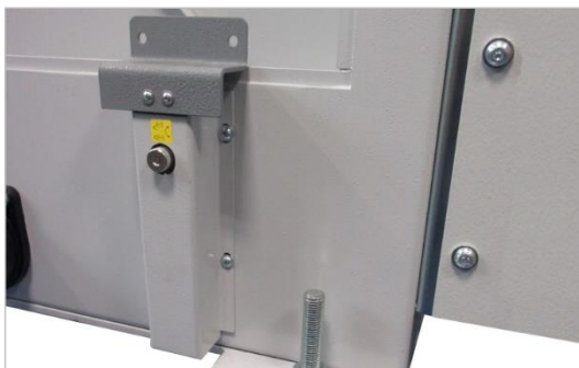
Figure 28: vertically mounted safety switch
