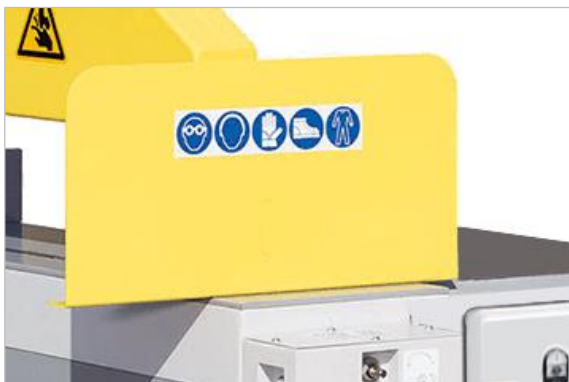
Figure 33: protective shield (standard version)
