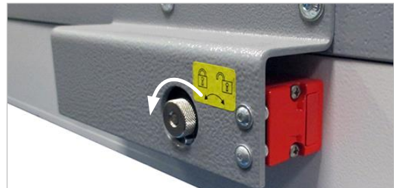
Figure 27: safety switch UTK 600 - door locked
