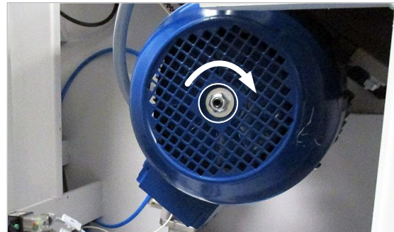
Figure 55: brake adjustment screw 5.5 / 7.5 kW
