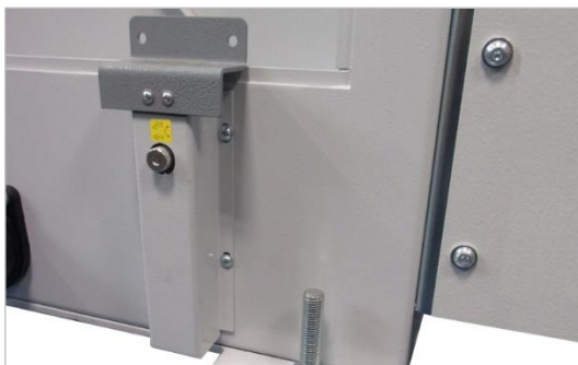
Figure 28: vertically mounted safety switch
