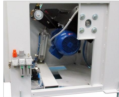
Figure 49: motor cover plate removed
