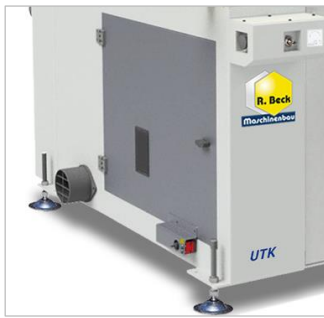
Figure 40: saw blade access door
