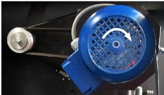
Figure 54: brake adjustment screw 2.2 / 3.0 / 4.0 kW
