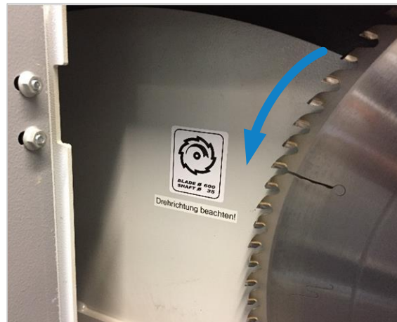
Figure 30: direction of rotation of the saw blade
