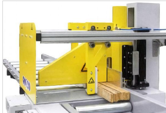
Figure 38: pneumatic horizontal clamping device
