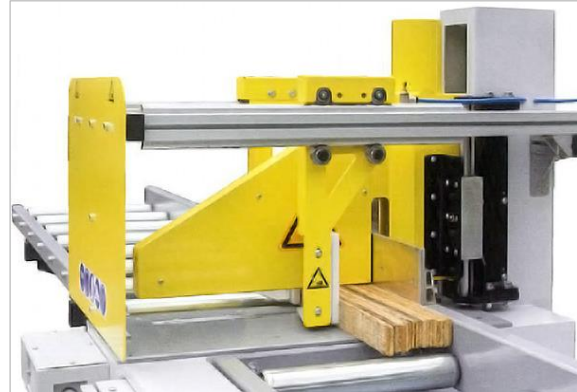
Figure 38: pneumatic horizontal clamping device
