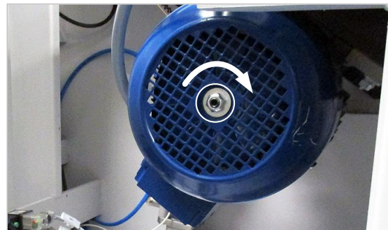
Figure 55: brake adjustment screw 5.5 / 7.5 kW
