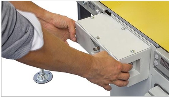
Figure 43: cut triggering via two-hand control
