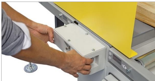
Figure 24: two-hand safety control
