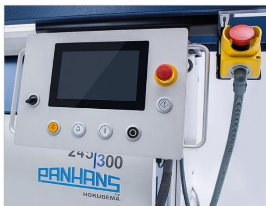
Figure 13: Emergency Stop Push Buttons
