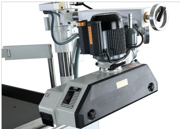
Figure 59: Power feeder type PV84
