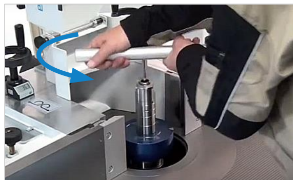
Figure 17: Loosen & remove the milling arbor with spanner
