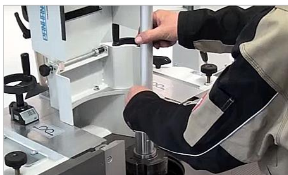
Figure 16 : retirer le cache-poussière
