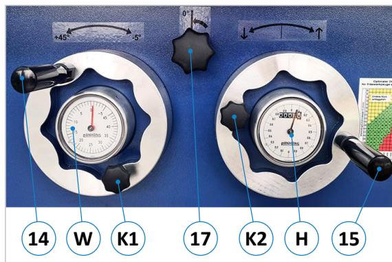
Figure 20: Handwheels for height / tilt adjustment
