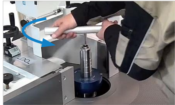
Figure 19: Loosen & remove the milling arbor with spanner
