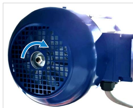
Figure 87: Adjusting screw of the motor brake
