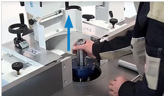
Figure 20: Remove milling arbor
