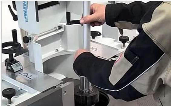
Figure 18: Remove dust protection cap
