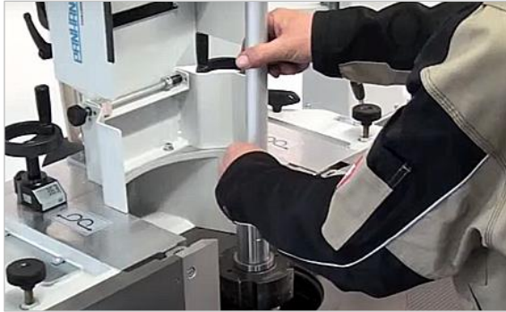
Figure 17: Remove dust protection cap
