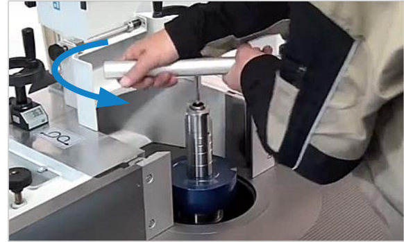
Figure 18: Loosen & remove the milling arbor with spanner
