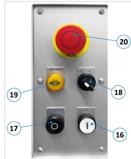
Figure 18: Control panel (fixed speed)
