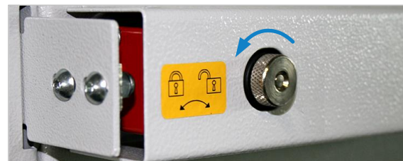
Figure 21: Safety switch - door locked
