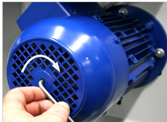
Figure 45: Readjusting the motor brake
