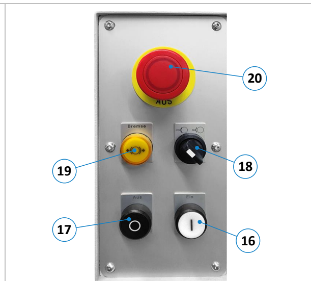
Figure 14: Control panel (fixed speed)
