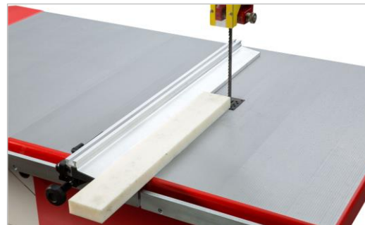
Figure 32: Fence turned to flat position
