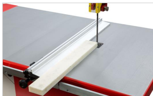
Figure 32: Fence turned to flat position
