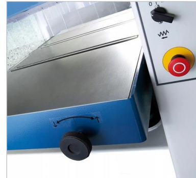
Figure 48: Adjusting the table rollers
