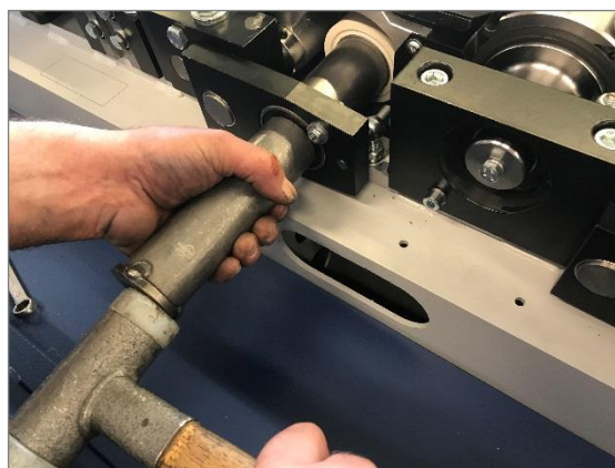
Figure 69: Rubber roller replacement Step 5b
