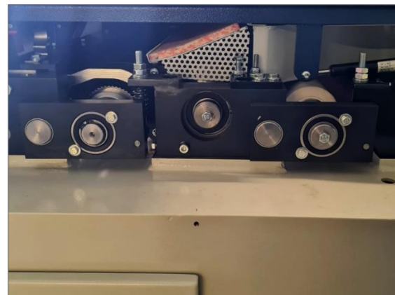
Figure 65: Rubber roller replacement Step 1b
