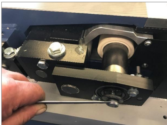
Figure 80: Rubber roller replacement Step 2
