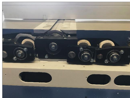
Figure 79: Rubber roller replacement Step 1b
