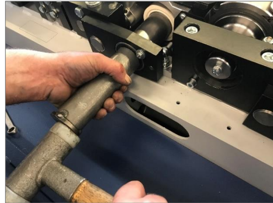
Figure 83: Rubber roller replacement Step 5b
