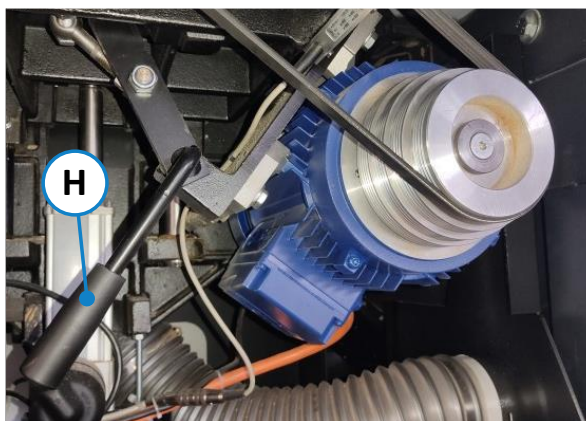
Figure 52: Speed setting - loosen V-belt
