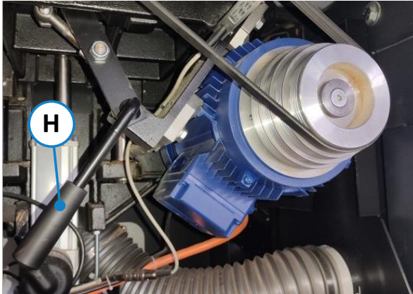
Figure 52: Speed setting - loosen V-belt
