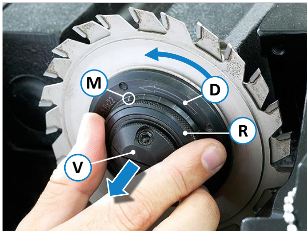
Figure 79: Quickstep setting mechanism for scoring saw blade
