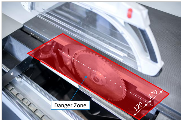
Figure 2: Danger zone saw blade
