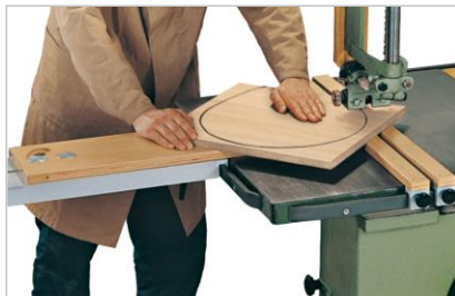
Figure 44: Kreisfix for circular cuts
