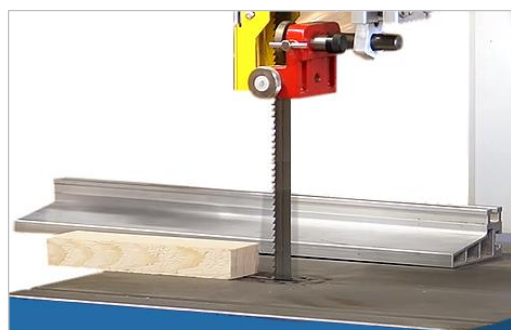
Figure 35: Fence turned to flat position
