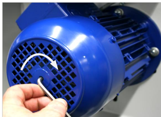
Figure 53: Readjusting the motor brake
