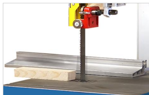
Figure 35: Fence turned to flat position
