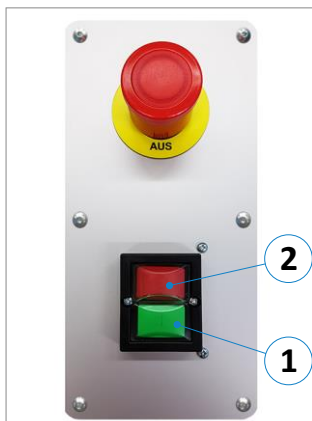
Figure 19: Push-button unit (1.1 - 1.5 kW)
