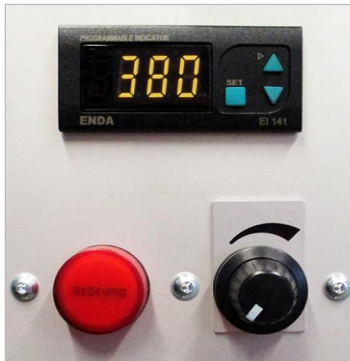
Figure 39: Blade speed control
