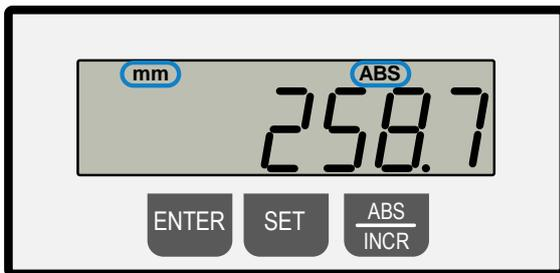
Figure 2: Display mode mm/ABS
