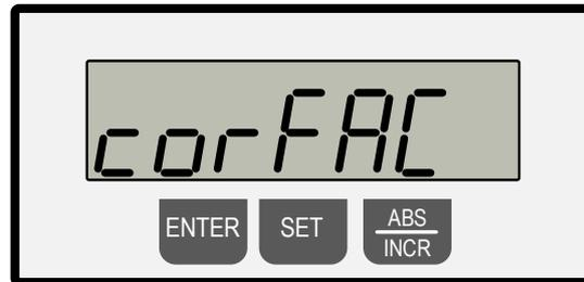
Figure 6: Change/enter calibration unit 2
