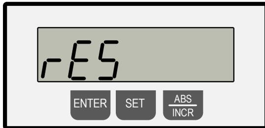
Figure 5: Change/enter calibration unit 1
