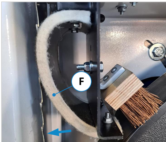
Figure 81: Felt for bandsaw blade lubrication
