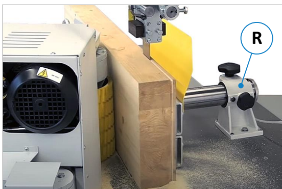
Figure 70: Roller fence and feed unit in use
