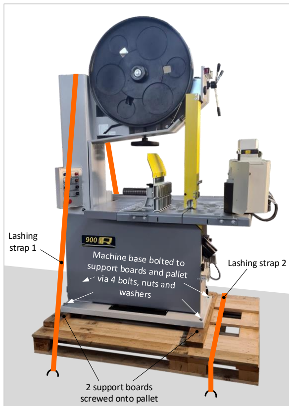
Figure 12: Lashing the machine
