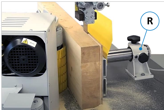
Figure 70: Roller fence and feed unit in use
