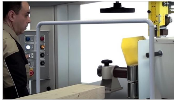
Figure 85: Switch on bandsaw drive and feed unit
