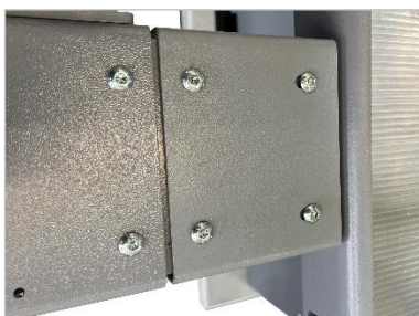
Figure 50: Bridge plate mounted
