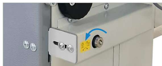
Figure 45: Safety switch - door locked
