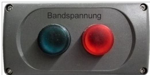
Figure 67: Visual saw blade tension monitoring
