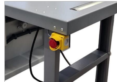
Figure 35: E-stop on removal table
