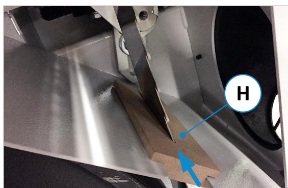
Figure 61: Attaching the suction aid board
