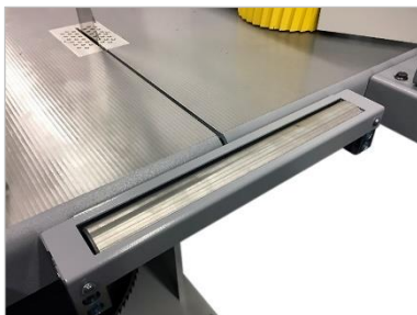
Figure 47: Conveyor roller mounted
