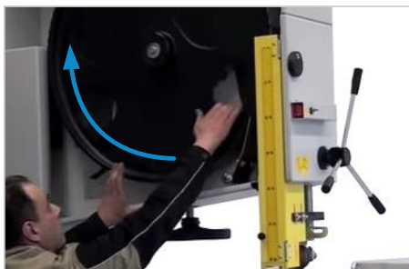
Figure 59: Adjusting the saw blade run
