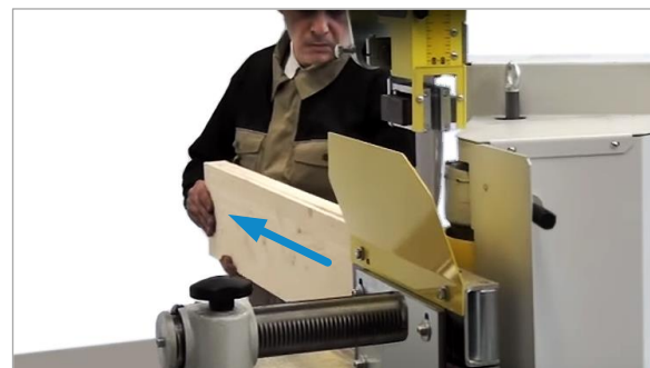
Figure 89: Remove workpiece parts on the removal side
