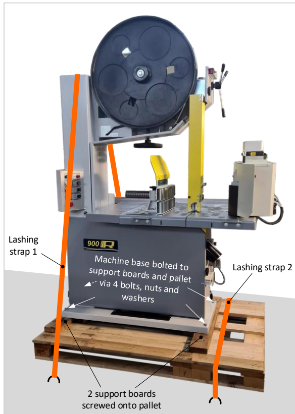
Figure 12: Lashing the machine
