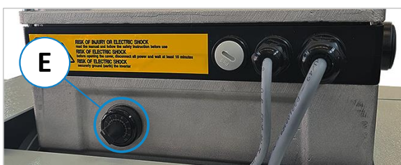
Figure 80: Setting wheel for variable feed rate
