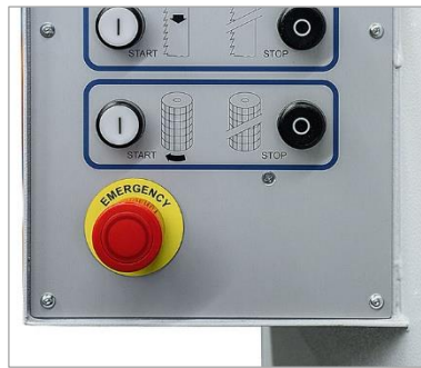
Figure 31: E-stop control panel
