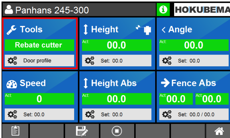
Figure 25: Open the tool and program memory in the machine overview
