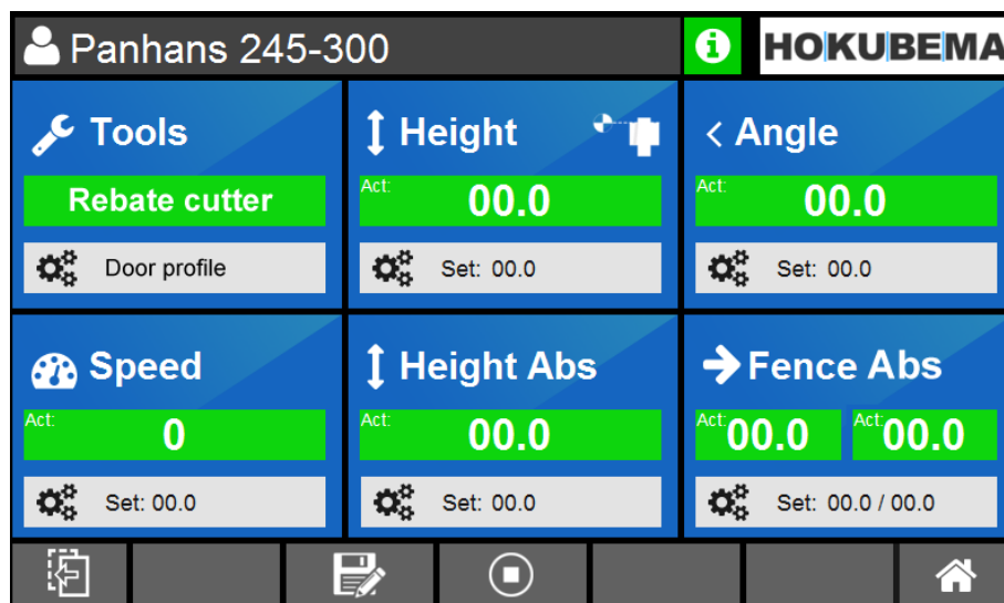
Figure 7: Machine overview mask with tools, axis positions and speed (example 245/300)
