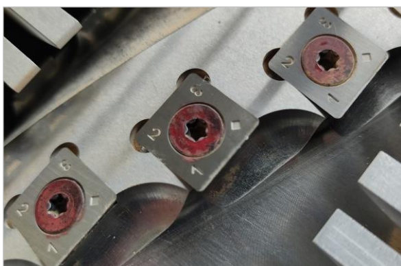
Figure 42: Indexable inserts of the spiral cutter block
