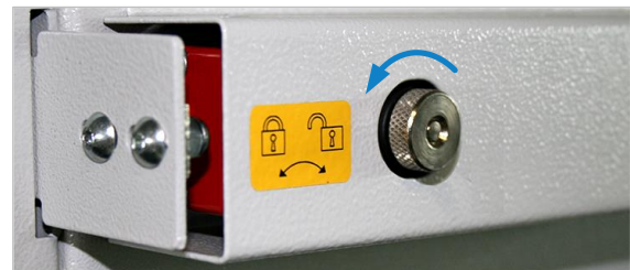
Figure 16: Safety switch - door locked
