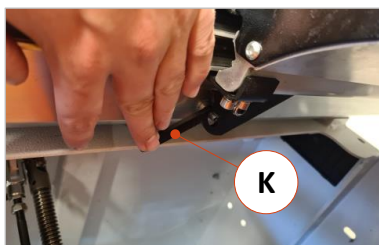
Figure 21: Press the safety catch
