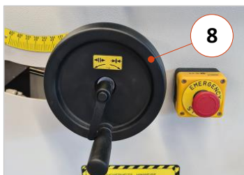
Figure 27: Tilt setting wheel
