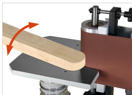
Figure 40: Sanding an outer radius
