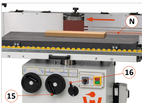
Figure 43: Sanding off veneer protrusions
