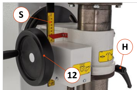
Figure 17: Height setting with handwheel and scale
