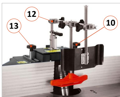
Figure 19: Standard safety fence
