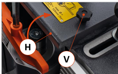
Figure 23: Fold up protective bonnet
