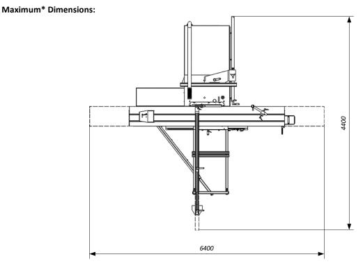
\*) Depending on the position of the sliding table and the cross-cut fence. The dimensions shown are rounded approximate dimensions.
