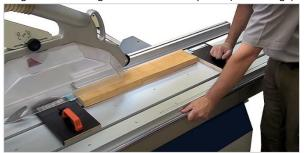
Fixing & cutting of very short and small workpieces:
