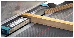
Fixing & damage-free cutting of smallest workpieces:
