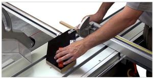
Make the cut by pushing the slide table forward:
