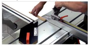
Slide Safety-Power via groove to the workpiece and fix it:
