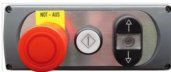
Figure 5: Two-hand control for height adjustment
