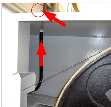
4. Guide the cable through the cable gland.
