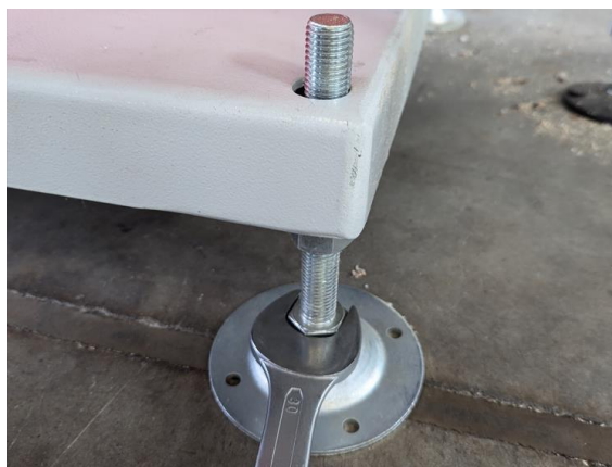
Figure 4: Levelling the machine
