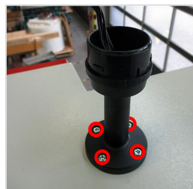
6. Mount the signal tower base on the hood using 4 screws.
