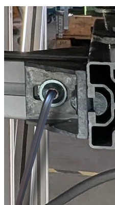
Figure 22: Mount connecting profiles (A) on the front and back of the profile (P)
