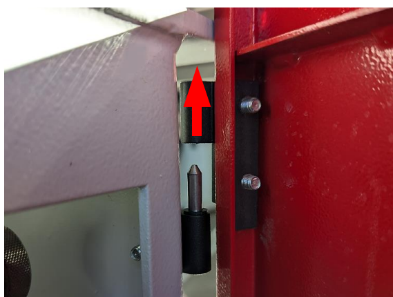
Figure 33: Remove lower bandsaw wheel door
