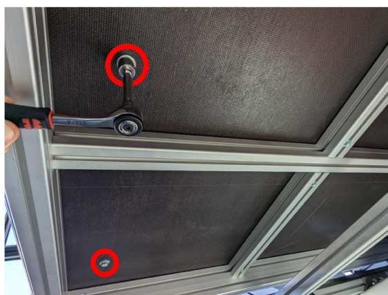
Figure 29: Adjusting the 90° angle of the lateral stop rail
