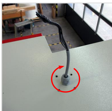
5. Tighten the cable gland on the top of the hood.
