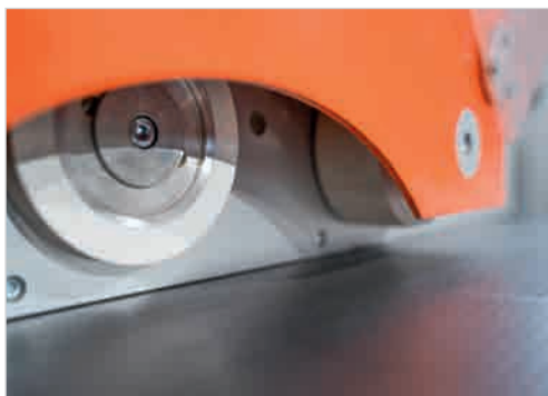
Circular saw feeder 76: Infeed roller in detail
